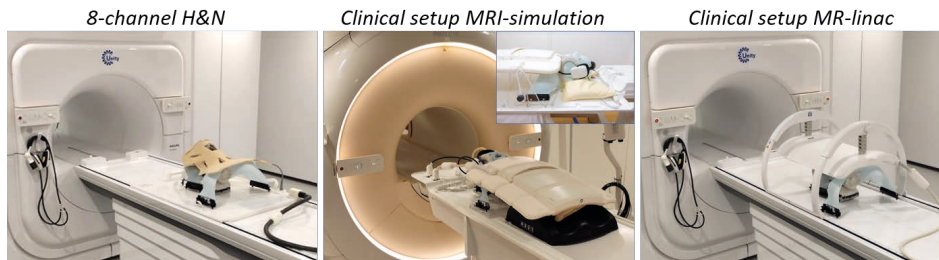
Figure 4.4 Imaging setups of the 8-channel H&N array (left), clinical MRI-simulation setup (middle), and clinical MR-linac setup (right). The imaging setups are shown on a phantom but data were acquired in-vivo.
