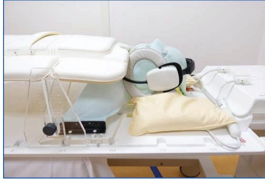
Figure 1.5 Clinical setup for MRI-simulation before H&N radiotherapy. The setup consists of two loop coils against the head and a 16-channel anterior element on a coil bridge that is placed against the chin.
