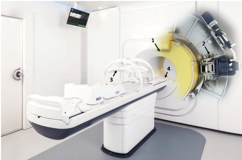
Figure 1.1 The 1.5 T Elekta Unity MR-linac. This hybrid machine combines an MRI scanner (1) and a linear accelerator (2). The MRI receive hardware consists of a 4-channel anterior element (3) and 4-channel posterior element that is located in the middle of the bore under the table (4). Image adapted from Elekta (2018).
